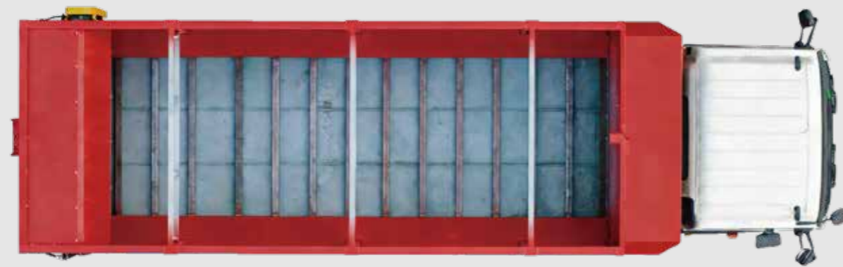
Chain Scraper Structure Inside the Hopper
