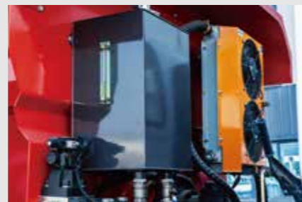
Hydraulic Oil Tank and Radiator System
