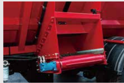
Discharge Control Gate
